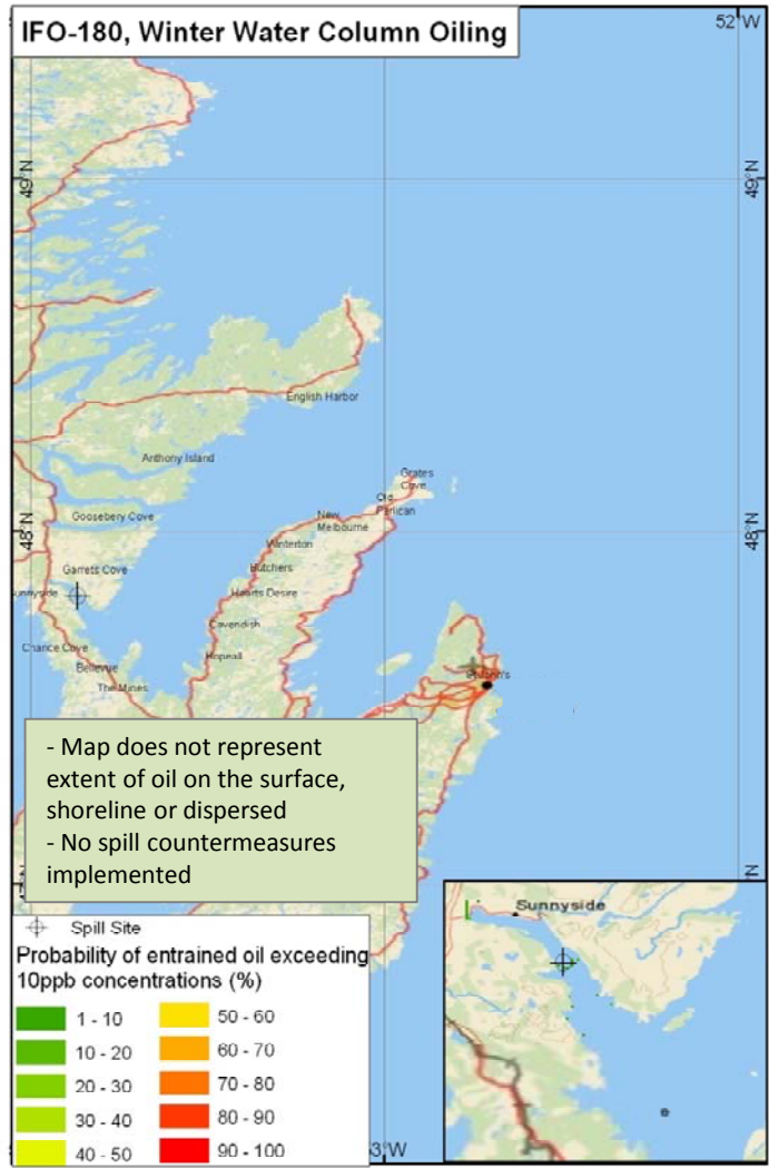
Figure B12. Probability of entrained oil from a release of 1,000 m 3 of Intermediate Fuel Oil (IFO-180) at the Bull Arm site in winter.
